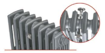
Wall stays provide a firm brace to the wall for your Cast Iron radiator. All our Cast Iron radiators are floor standing and stable, however, due to their weight, we strongly recommend you tie your radiator to the wall with wall stays for added safety.
