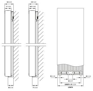
Connections Each radiator comes with 1/2'' inlet connections as standard.
